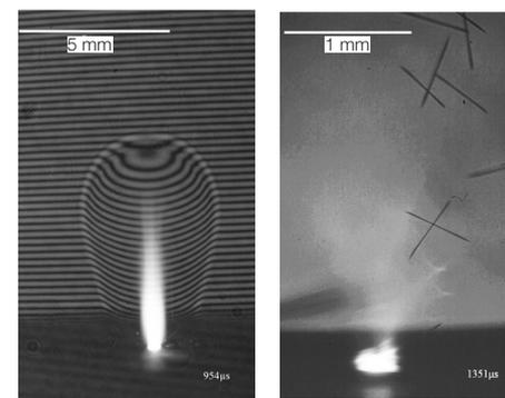
*High-speed interferometry (left) of the evolution of gas from a laser irradiated composite and nanosecond shadowgraphy (right) of ejected carbon fibres.*
