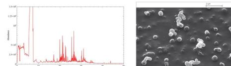
*Isokinetic gas sampling of laser-produced fume with the corresponding mass spectrum and captured particles.*
