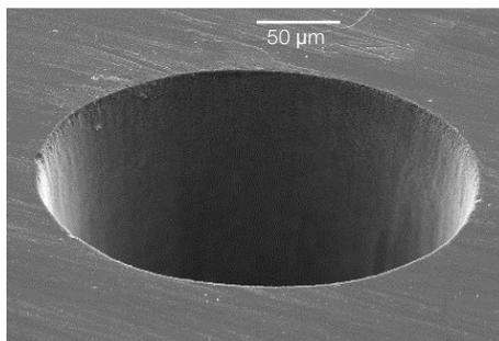
*Crack-free femtosecond laser trepanning of a hole in glass*
