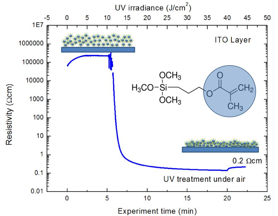
Fig. 1: Resistivity dependence on UV treatment of wet deposited ITO coating
