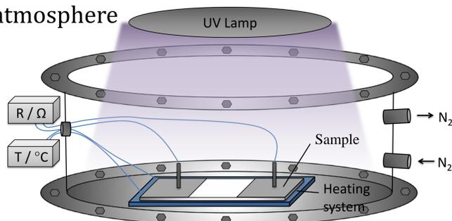
Fig. 2: In situ sheet resistance measurement system during UV treatment
