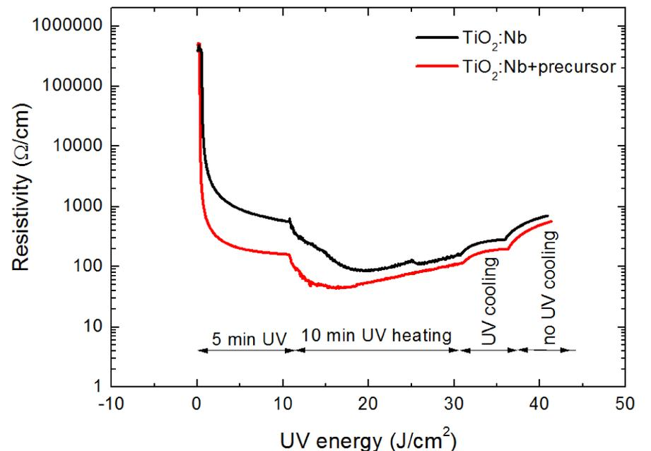
Fig. 4: Resistivity dependence on UV treatment of  $\text{TiO}_2\text{:Nb}$  inks
